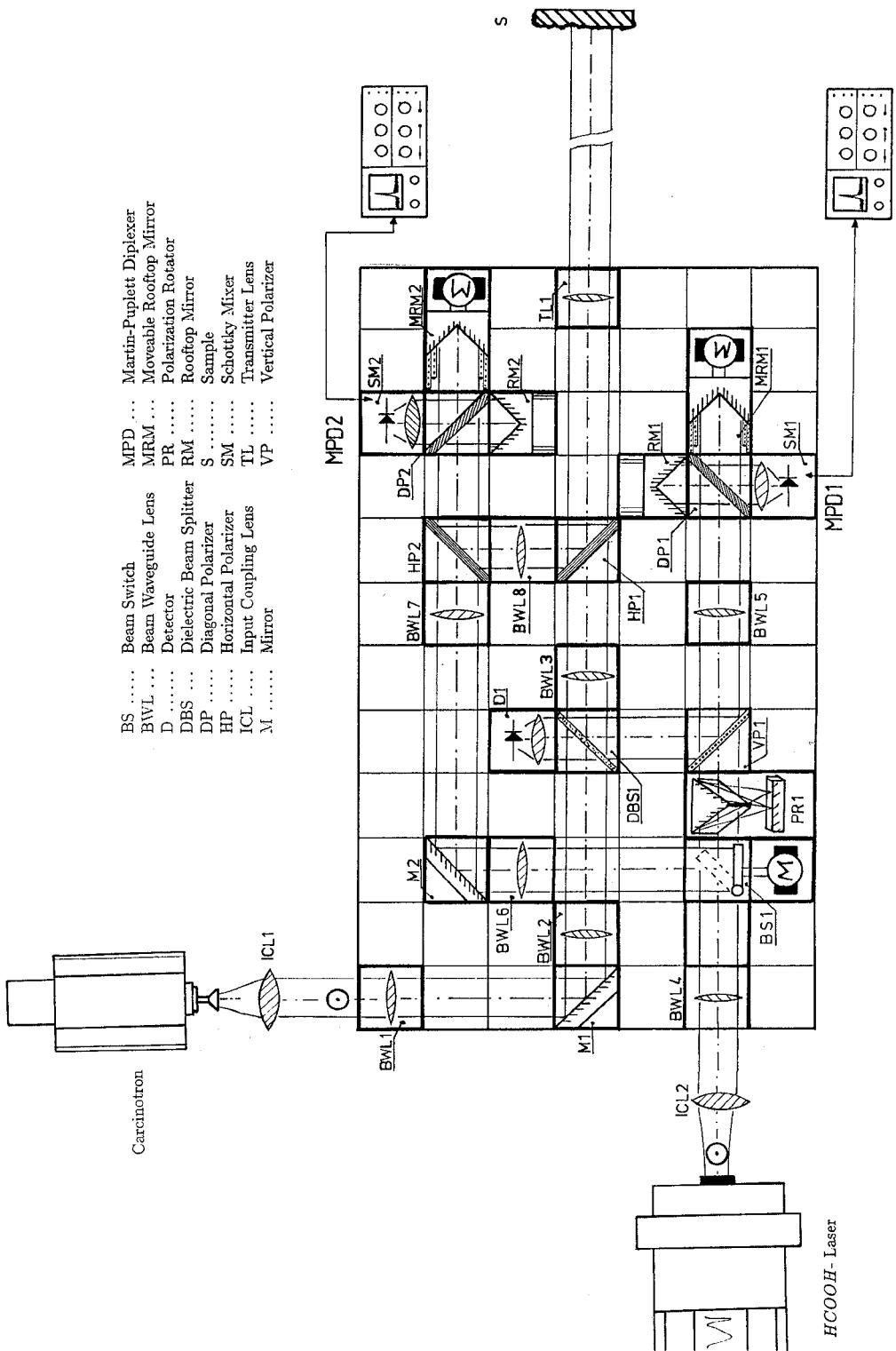
Figure 1: Principle of the polarimetric heterodyne reflectometer
